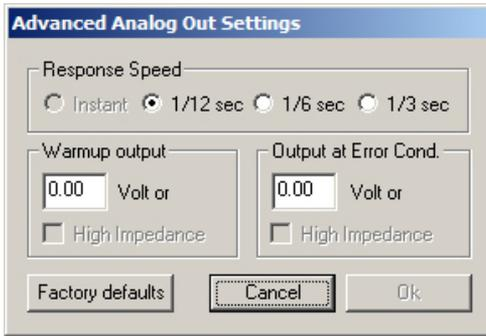
When setting the PSB-1 to the slower response speed settings, the measured mixture data will be averaged over the response time setting before being sent via the analog output.
