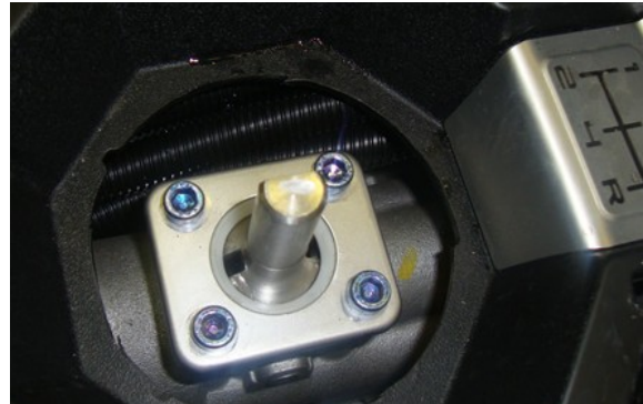
Plate installed ready for the boot to go back on
