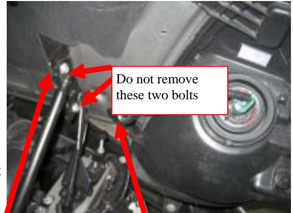
Remove these two plastic retainers
