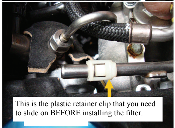
Push in with the GM fuel disconnect tool and pull back on the supply line at the same time.
