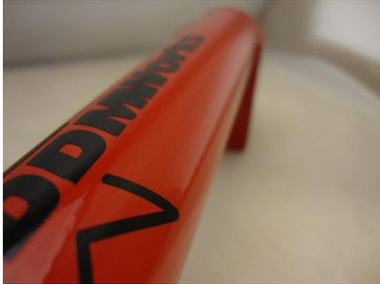
This front chassis brace is designed to add some stiffness to the chassis to help improve cornering stability and speed.
