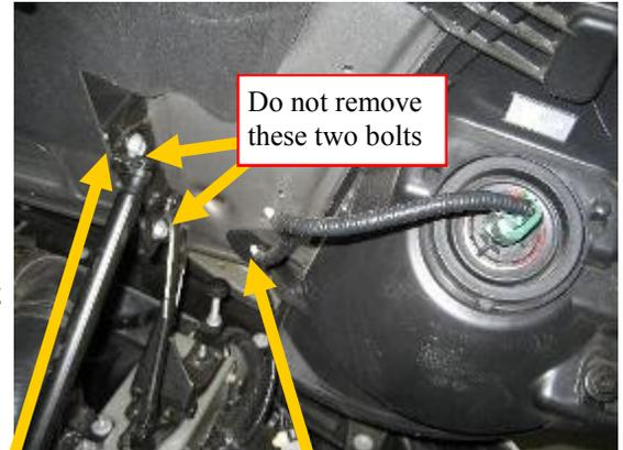
Remove the 2 nuts holding the hood directly to the metal bracket.
