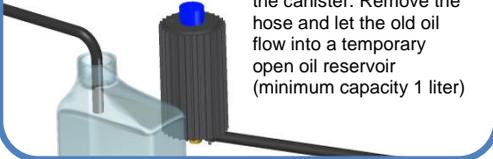
6. Remove the top banjo bolt and sealing washers on the canister. Remove the hose and let the old oil flow into a temporary open oil reservoir (minimum capacity 1 liter)
