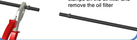
2. Slide away the two hose clamps on the oil filter and remove the oil filter
