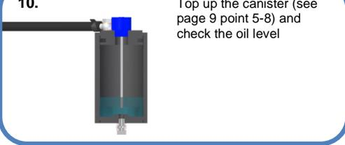
10. Top up the canister (see page 9 point 5-8) and check the oil level
