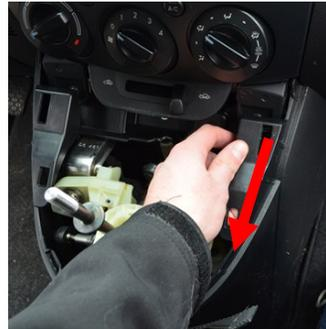
5. Now you can remove the four 12mm nuts which hold the shifter assembly in place, and remove the assembly from the mounting studs on the car.
