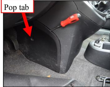
3. Next you need to remove the side panels for the lower dash. This is done by pulling out a pop tab in the middle of the panel, then using a flat head screw driver to pull the rear part of the panel outwards. It will pop once loose. Once the rear of the panel is loose it just needs to be slid back to remove it. The panel on the driver side and passenger side both need to be removed.
